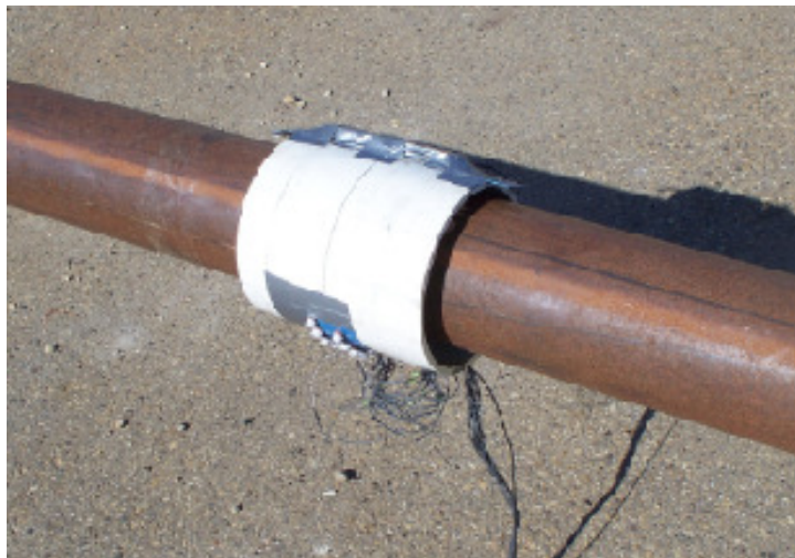
Figure 2. A 16-channel prototype TT probe for testing 6" carbon steel pipe.
