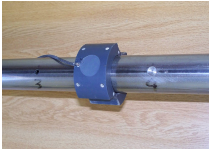
Figure 1. A 5-channel TT probe for testing a \phi 1.75 " carbon steel tube.
